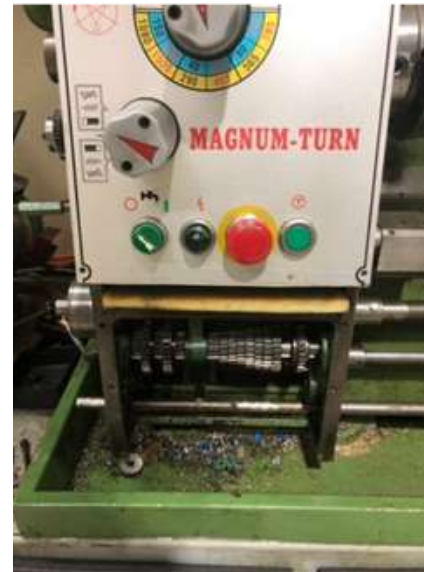
Feed gearbox under repair
