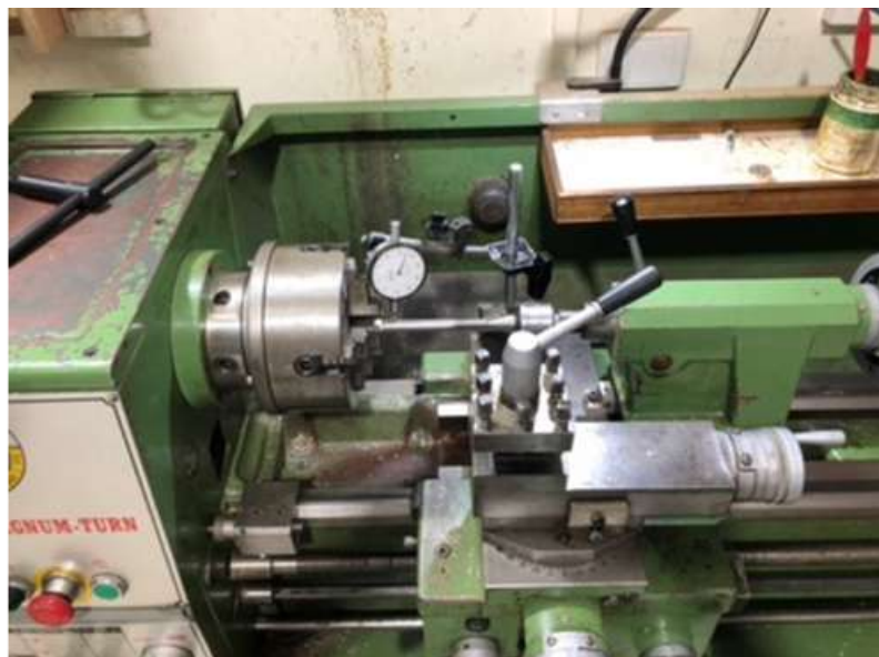
Four jaw chuck being set up with dial indicator
