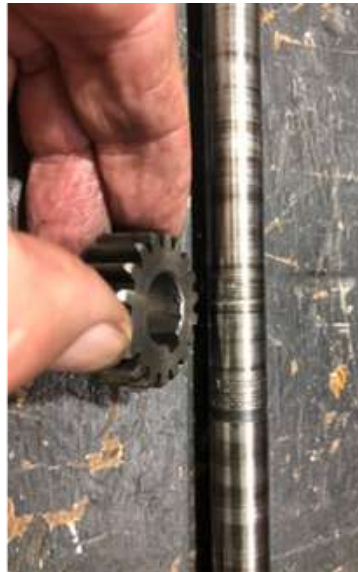
Damaged selector shaft
