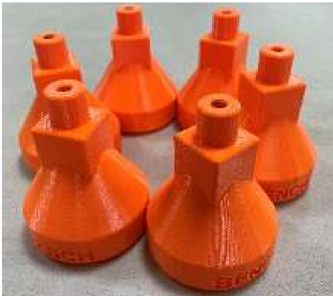
The 3D printer has had a workout making feet for the new multi-function tables (MFT) for the workshop.
