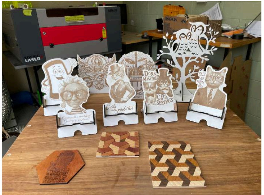
This group is experimenting with different materials to produce various items. The Laser can make boxes, phone holders and even inlays.
